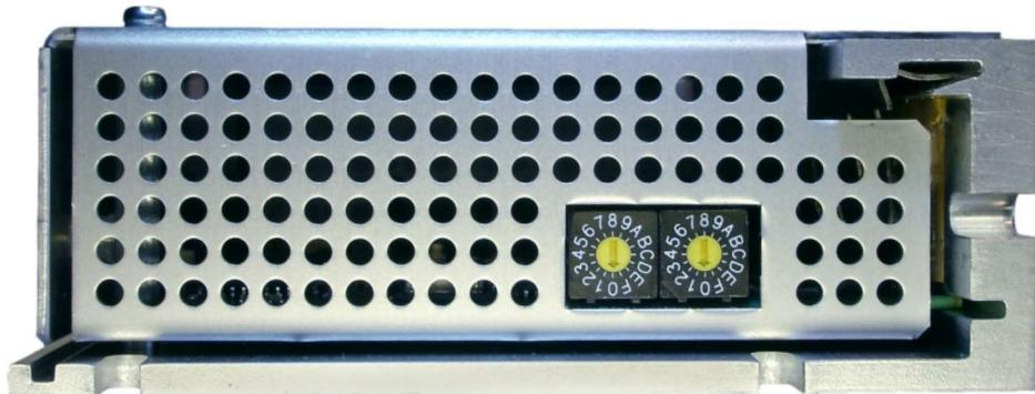
The address is set in hexadecimal format. For an address up to 15, the left-hand rotary switch remains at zero. For higher addresses, the left-hand rotary switch position is multiplied by 16 and added to the right-hand value.
