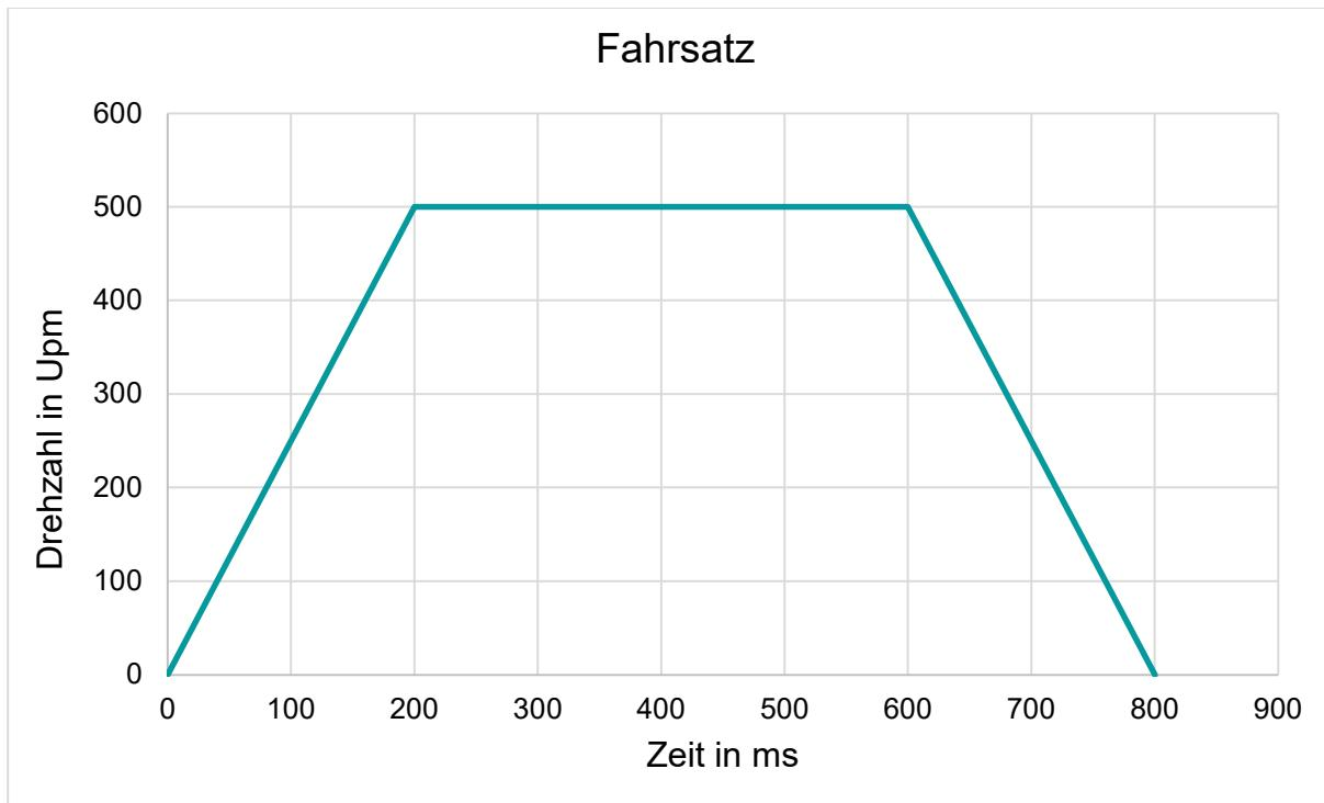
*Like the braking time, the acceleration time is 200 ms.
