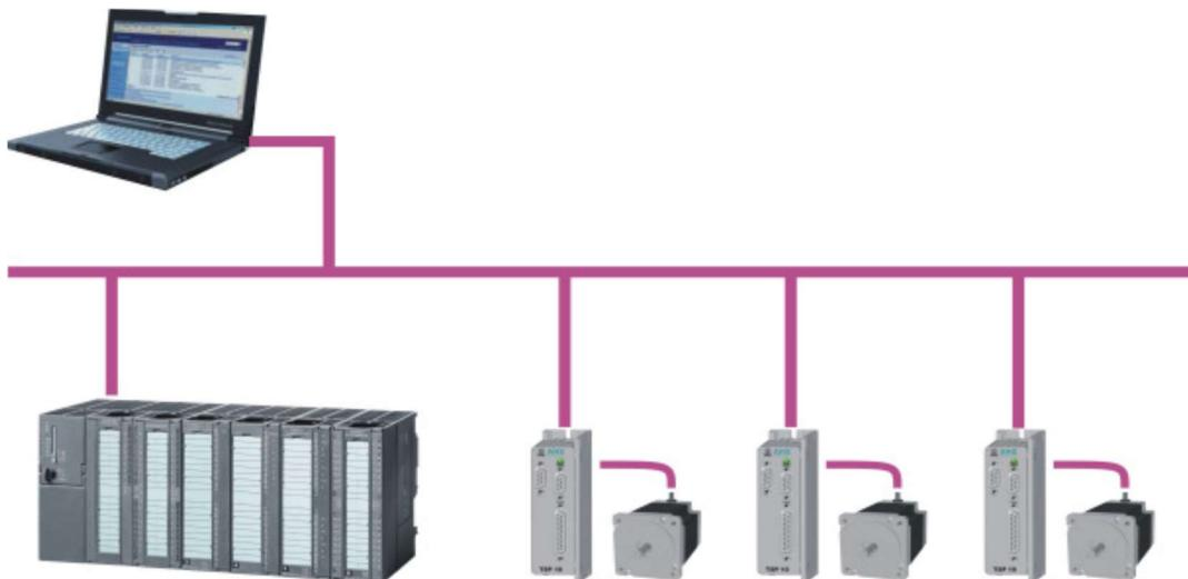
The current status and position can be recorded by the control at any time by reading the input data.
