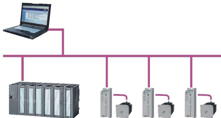
The CANopen step motor drive is a compact single-axis positioning controller with integrated stepper motor output stage. It detects two limit switches, a stop switch and a reference switch. The speed mode and the positioning mode can be easily configured via CANopen.
