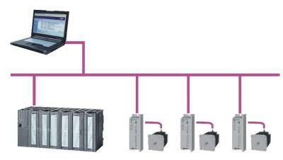
The Profibus DP Stepper is a compact single-axis positioning controller with integrated stepper motor output stage. It detects two limit switches, a stop switch and a reference switch. The speed mode and the positioning mode can be easily configured via the Profibus.
