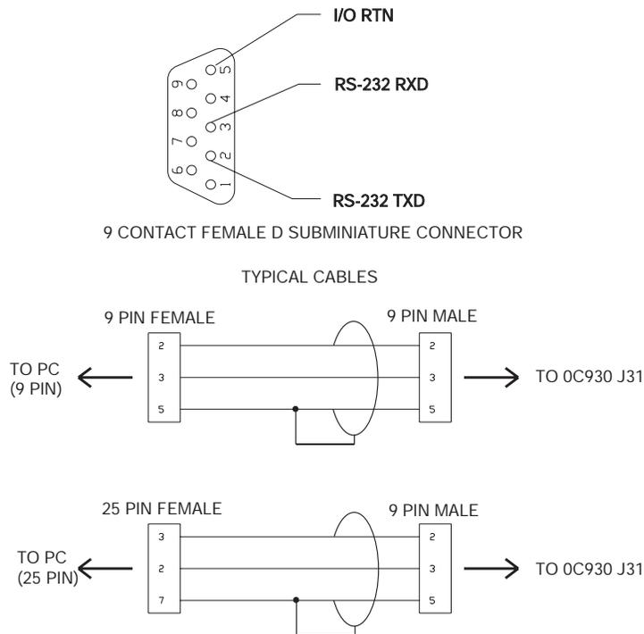
**Note:** *Shielded wiring is recommended for the serial communications cable to minimize potential errors from electrical noise.*
