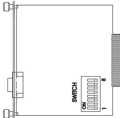
The diagram below shows the S1 default switch settings. The OC930 factory default address is 255.
