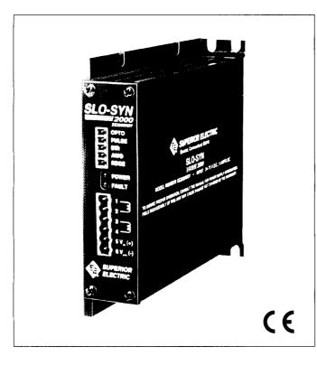
The SS2000MD7 is the ideal solution for cost effective modular drive systems. Modular drives are well suited for multiple axes applications because they can be operated from one power supply. The SS2000MD7 drive is a bipolar PWM drive, a design which provides maximum torque over a wide range of speeds and is suitable for 4-, 6- or 8-lead motors.
