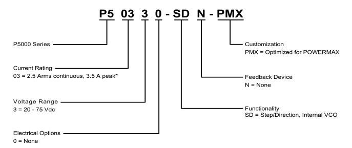
\*Note: Switch selectable in 0.2 Amp increments, 0.7 - 3.5 A
